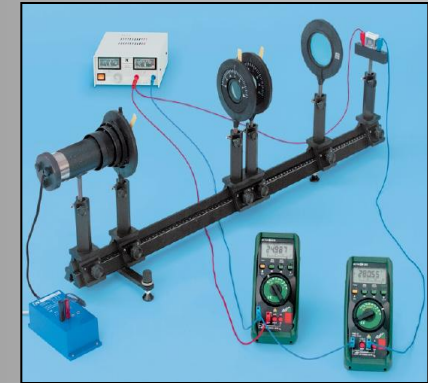
Recording the current-voltage characteristic of a CdS photoresistor
