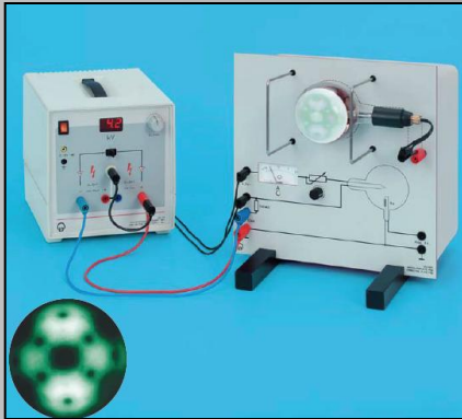
Investigating the crystal structures of tungsten using a field emission microscope
